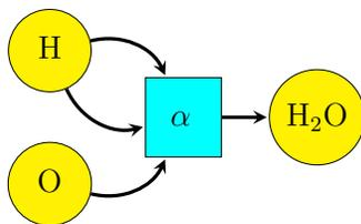
Here we have a set of ‘places’ (or in chemistry, ‘species’) drawn in yellow and a set of ‘transitions’ (or ‘reactions’) drawn in blue. The disjoint union of these two sets then forms the vertex set of a directed bipartite graph, which is one description of a Petri net.
