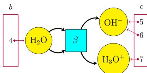
Since the outputs of the first open Petri net coincide with the inputs of the second, we can compose them by identifying the outputs of the first with the inputs of the second:
